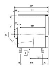
Drain Electrical inlet (power)
